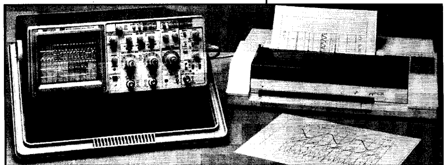
For convenient documentation you can link the 2211 or 2201 to a 4-color plotter such as the HC100, to print the waveform record.
